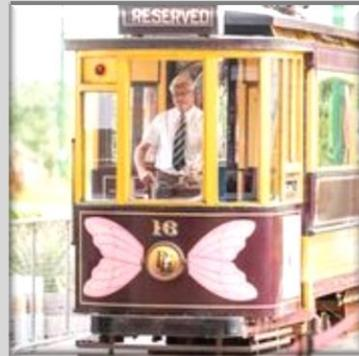
**Type:** Bogie, single deck, fully enclosed. Based on the Bournemouth open top tramcar cut to a single deck. Rebuilt at Seaton between 1974 and 1991.
