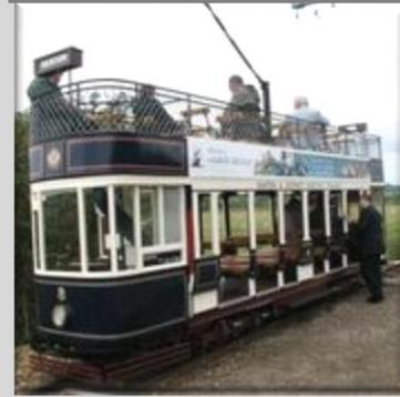
**Type:** Bogie, double deck open top, lower deck open cross bench design with small saloons. Based on the ex-Bournemouth open toppers of the Llandudno & Colwyn Bay system. Was the first car to be built for the Seaton gauge of 2', 9".
