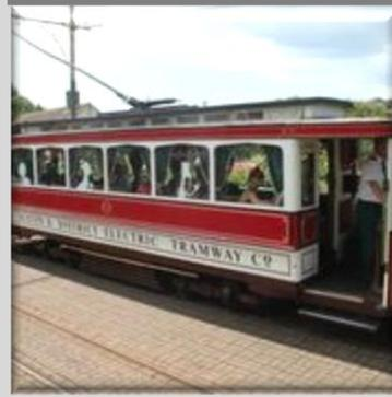
**Type:** Bogie, single deck, fully enclosed
