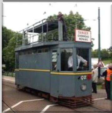
**Type:** Four wheel totally enclosed car, then bogie totally enclosed with overhead platform. Is usually found at the Riverside Depot and is used for maintenance of the track.
