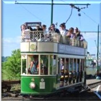
**Type:** Bogie, double deck open top, lower deck open cross bench design. Based on the ex-Bournemouth open toppers of the Llandudno & Colwyn Bay system.
