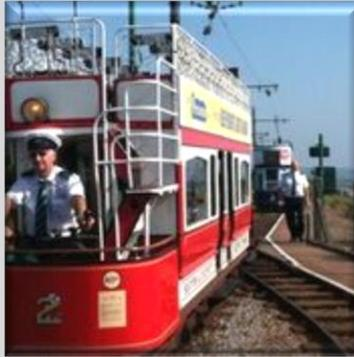
**Type:** Bogie, open top, uncanopied double deck
