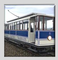
**Type:** Bogie, single deck, open cross bench. Based on the Manx Electric Railway toast-rack cars. Was re-built in 2016 as an enclosed saloon. Used to be car 17.
