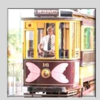
Type: Bogie, single deck, fully enclosed. Based on the Bournemouth open top tramcar
