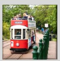
**Type:** Bogie, single deck open top, fully enclosed, later double deck, open top. The rebuild of 1999, based on the London Feltham trams of the 1930's. The most rebuilt tram in the fleet.
