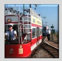
Type: Bogie, open top, uncanopied double deck
