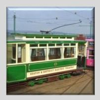
**Type:** Bogie, single deck totally closed. Based on the Exeter open top tramcar cut to single deck. Was an Exeter Corporation Tramways 3'6" gauge open topper from 1906 until 1931. It was rebuilt at Seaton between 1994 and 1998 and is the only Exeter Tram in preservation.
