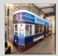
**Type:** Bogie, double deck open top, drop centre lower deck. Hybrid design based on elements of the old Plymouth and Blackburn trams.
