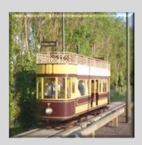
Type: Bogie, double deck open top, lower deck open cross bench design. Based on the
