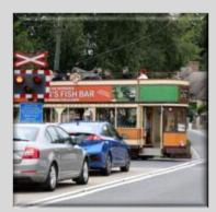
**Type:** Bogie, double deck open top, drop centre lower deck. Hybrid design based on elements of the old Plymouth and Blackburn trams.
